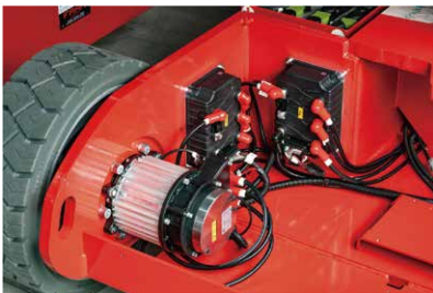
Permanent magnet drive (Standard)
