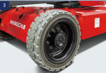
Tires: foam-filled tires with good off-road performance
